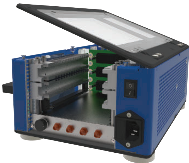
The Elma small portable OpenVPX development platform is designed to help engineers build next-generation high-throughput embedded computing systems.
