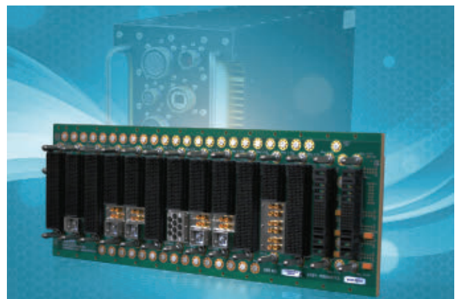
This photo shows an aperture design approach for backplanes and chassis that enables designers to blend optical and copper point-to-point interconnects in the same system.
